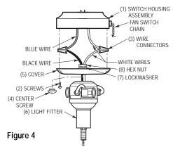
6. Connect the white wire from the ceiling fan to the white wire of the light kit fitter(6). Connect the blue wire from the ceiling fan to the black wire of the light kit fitter. Use listed wire connectors(3) (previously removed in step 3) to make connections. (Figures 4 and 5.)
